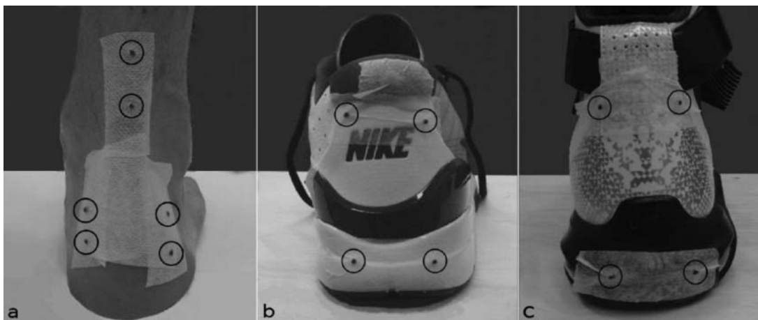
Figure 1. Location of beads on the rearfoot and shoes used to measure relative motion.
